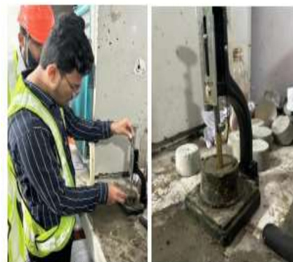
Fig 19 Testing for Consistency of Cement
