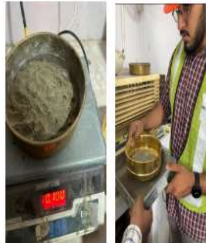
Fig 20 Testing for Fineness of Cement
